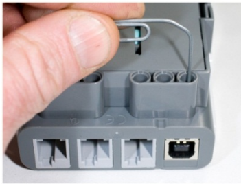
Figure 4: Location of the reset button to return NXT brick to factory settings.
