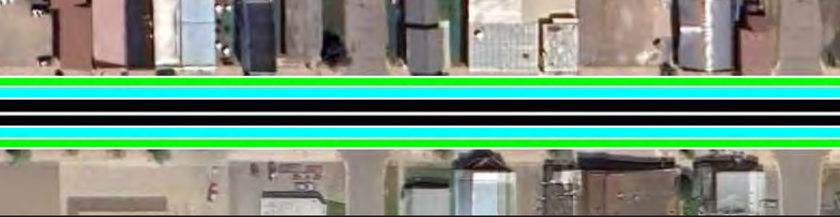
Above: Reducing the width of the travel lanes will slow traffic and provide space to consider angled parking or bike lanes (blue) and street trees, planters, bioswales, benches, etc. (green).
